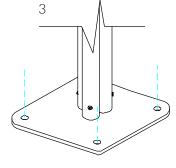
Fix Surface Plate to the ground surface Ground Anchors Not provided cover fixings with caps provided
